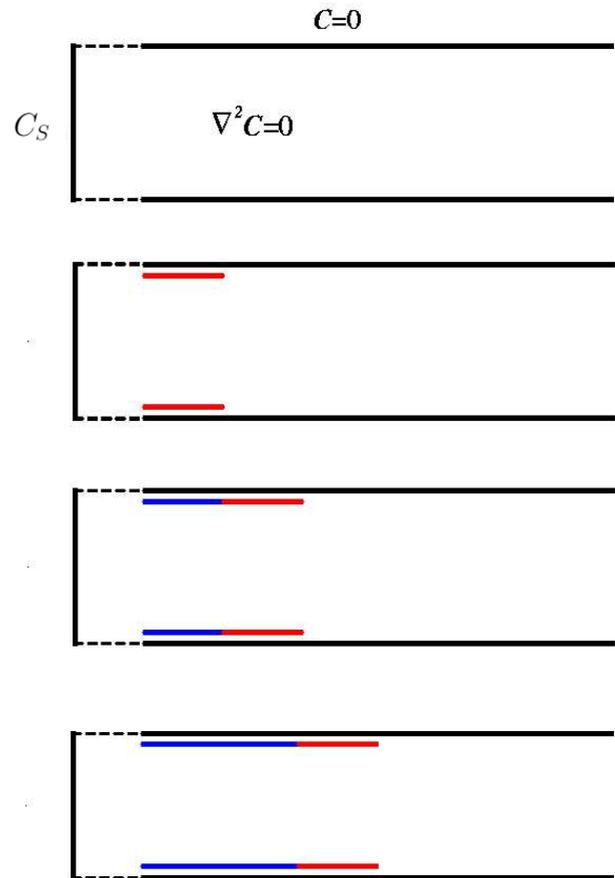
**Fig. 2** Schematic diagram of the passivation process applied to a smooth pore. The amount of the interface  $L_{it}(p)$  which is passivated (shown in red) at each iteration of the process remains constant. It is of the order of half the entrance diameter  $L$ . The passivation process follows as a simple sequence of translations of the pore inlet by the same passivated distance (shown in blue)  $L_{it}(p)/2$ .
