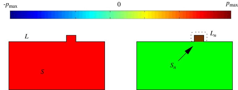
Fig. 6. Simplified explanatory scheme for the different dissipation properties of a localized and a non-localized mode in an irregular cavity (Color online).
