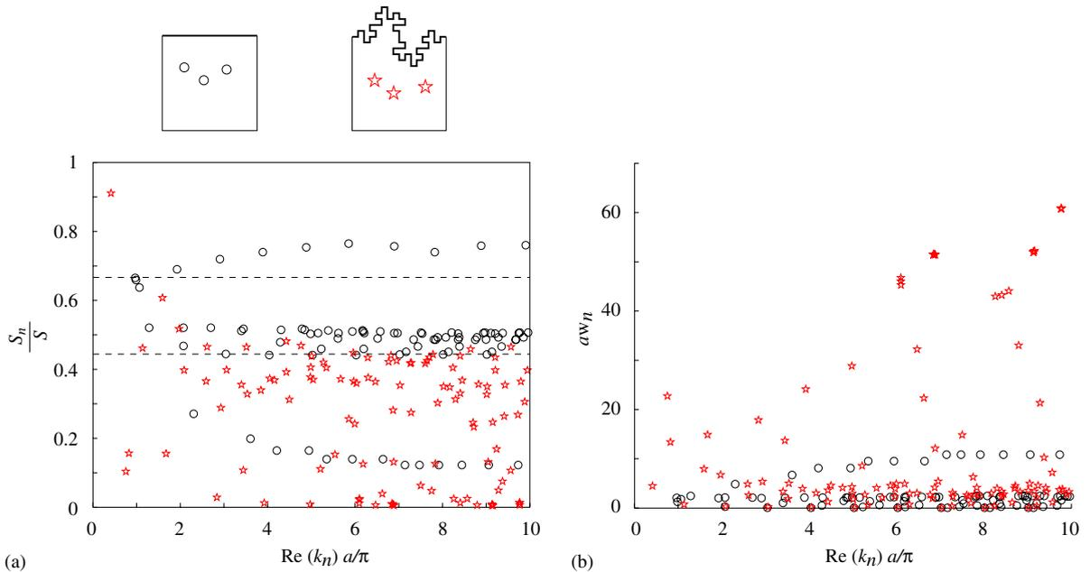
Fig. 8. (a) Relative existence surface and (b) energy dissipation, as measured by  $w_n$  (normalized by  $1/a$ ), for the first eigenmodes ( $\text{Re}(k_n)a/\pi \in [0, 10]$ ) of the cavities shown in insets, of which the upper boundary admittance is lined with a porous layer. The dashed lines on plot (a) indicate the possible values for a lossless square cavity (Color online).
