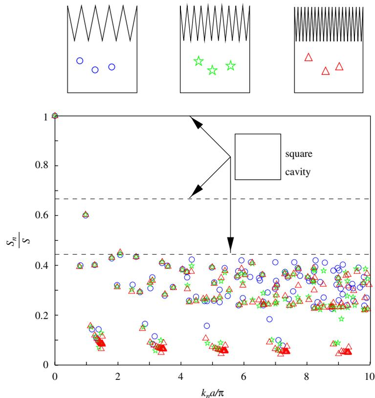
Fig. 2. Relative existence surface of the first eigenmodes ( $k_n a/\pi \in [0, 10]$ ) of the cavity of type (a) (see Fig. 1) with (○) 5; (✱) 10 and (△) 20 wedges, respectively. The dashed lines indicate the possible values for a square cavity. One observes that the more irregular the boundary the more localized the eigenmodes (Color online).
