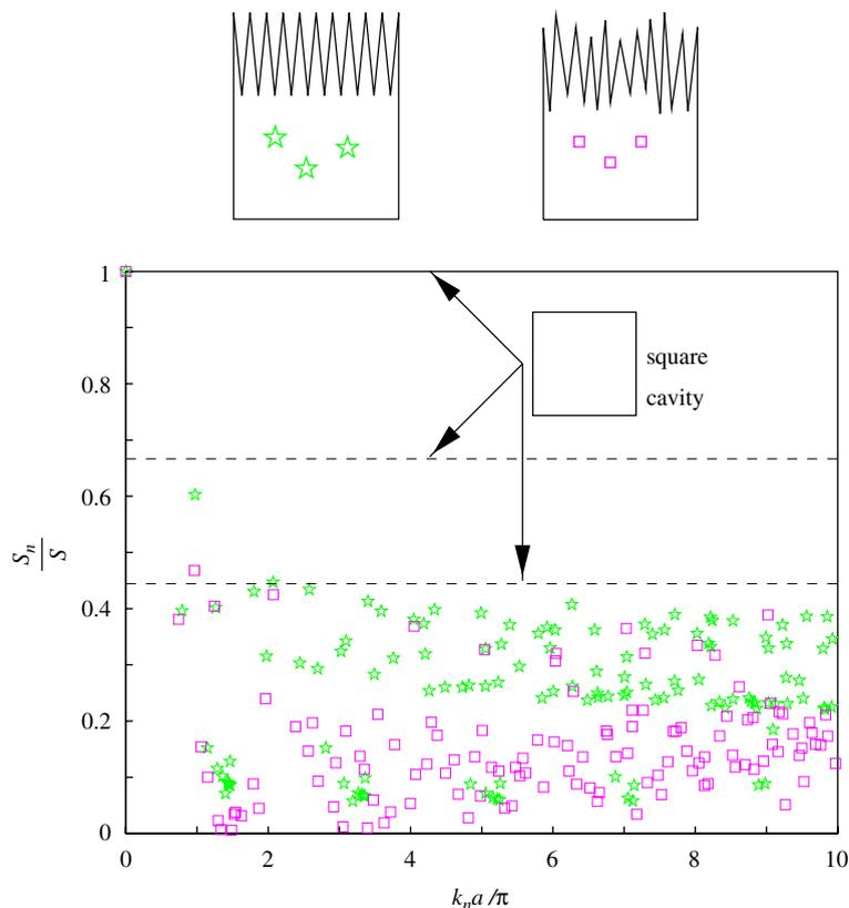
Fig. 3. Comparison between “regular” and randomized geometric irregularities, here a random set of wedges. The figure gives the relative existence surface of the first eigenmodes ( $k_n a / \pi \in [0, 10]$ ) of two cavities of identical surface area and perimeter length: ( $\star$ ) cavity of type (a) (see Fig. 1) with 10 identical wedges, ( $\square$ ) cavity of type (b) with 10 “disordered” wedges. The dashed lines indicate the possible values for a square cavity (Color online).
