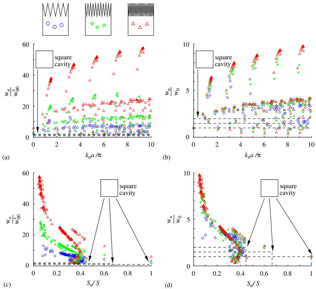
Fig. 7. (a) Energy dissipation, as measured by  $w_n/w_{00}^s$ , for the first eigenmodes ( $k_n a/\pi \in [0, 10]$ ) of the cavity of type (a) (see Fig. 1) with (○) 5, (✱) 10 and (△) 20 wedges, respectively. (b) same results, with  $w_n$  normalized by  $w_0 = L/S$  for each cavity, in order to emphasize the specific role of the localization. (c–d) Energy dissipation vs. the relative existence surface. The dashed lines indicate the possible values for a square cavity (Color online).
