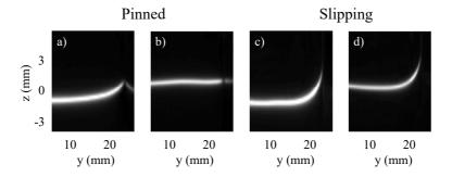
Figure 3. Transverse profile in the meniscus zone for  $\omega = 4\pi$  s<sup>-1</sup> and W = 42 mm. a) Wave trough with pinned contact line; b) Wave crest with pinned contact line; c) Wave trough with slipping contact line; d) Wave crest with slipping contact line. In this case z = 0 corresponds to the still water level without waveguides.
