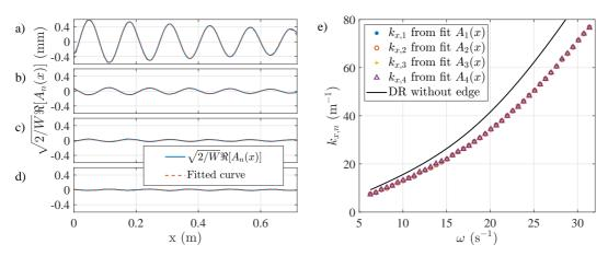
Figure 6. Longitudinal functions  $A_n(x)$  (real part) and fitted linear wave for the case W=22 mm and  $\omega=24.5 \text{ s}^{-1}$ . Panels a), b), c), and d) correspond to the functions  $A_1(x)$ ,  $A_2(x)$ ,  $A_3(x)$  and  $A_4(x)$  respectively. e) Fitted wavenumber  $k_{x,n}$  from the longitudinal functions  $A_n(x)$  with n=1,2,3,4 as a function of frequency.
