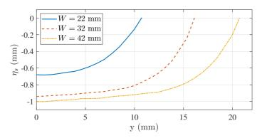
Figure 4. Static meniscus measured experimentally for three different channel widths. The vertical axis is shifted to set the contact line at z = 0.
