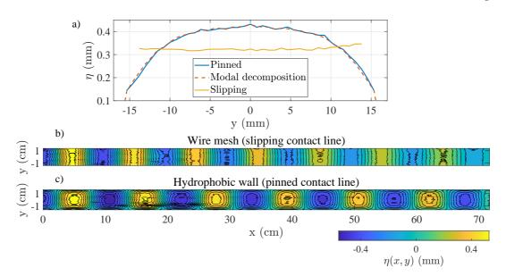
Figure 5. FTP measurements of the propagation of waves with slipping and pinned contact line conditions. a) Transverse profile of the surface perturbation ( $\omega = 8\pi \text{ s}^{-1}$ ; W = 32 mm; x = 0.6 m). b) Wave field with slipping contact line ( $\omega = 8\pi \text{ s}^{-1}$ ; W = 32 mm; Wavemaker phase  $\omega t = 3\pi/2$ ); c) Wave field with pinned contact line ( $\omega = 8\pi \text{ s}^{-1}$ ; W = 32 mm; Wavemaker phase  $\omega t = 3\pi/2$ ).
