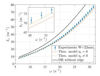
Figure 8. Theoretical dispersion relation for the case W=22 mm considering the relative contribution of measured meniscus  $\eta_s$ . Dotted line indicates the case  $\eta_s=0$ , dashed line shows the case  $\eta_s\neq 0$  (experimentally measured) and solid line shows the dispersion relation of water waves without edge constraints.
