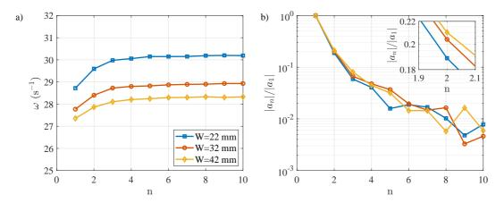
Figure 7. Three experiments at the same wave number  $k_x = 71 \text{ m}^{-1}$  and three different channel widths. a) Frequency  $\omega$  as a function of n calculated from eq. (20). b) Coefficients  $a_n$  obtained from the expansion of eq. (12) and the fit of eq (17), normalized by the first mode  $a_1$ . The inset shows a zoom over the mode n = 2.
