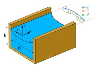
Figure 1. Coordinate system of the rectangular channel for the propagation of surface waves with pinned contact line
