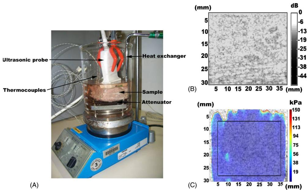
**Figure 1.** (A) Experimental set up. (B) Typical B-mode image. (C) Typical stiffness map and region of interest chosen for the shear modulus calculation.
