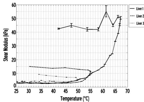
**Figure 2.** Evolution of the shear modulus with temperature for three samples extracted from one bovine liver. Error bars represent the spatial variance of the shear modulus in the ROI.
