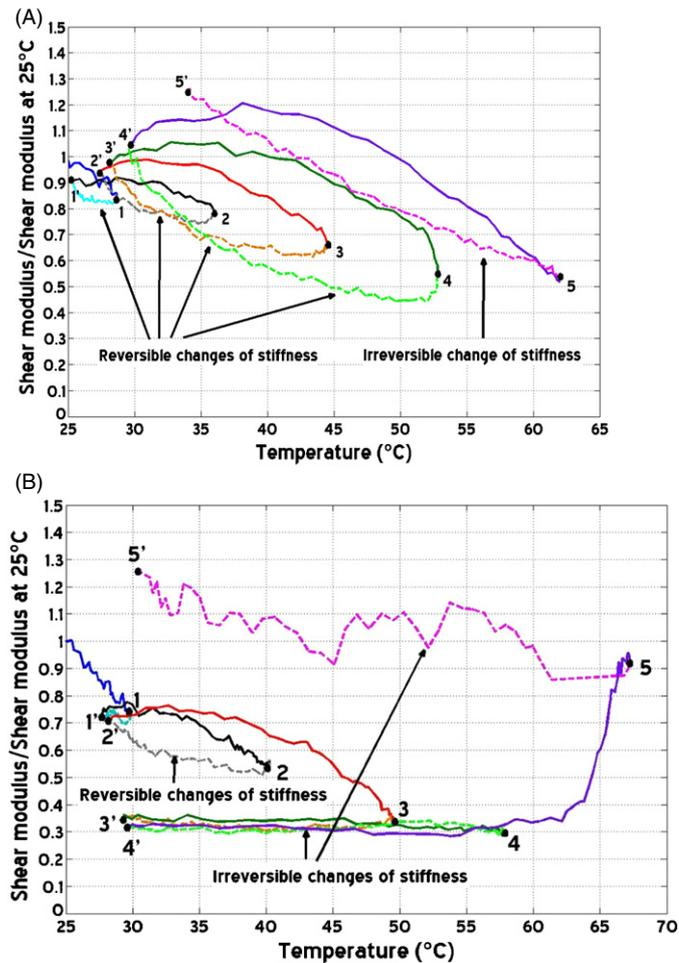
**Figure 6.** Evolution of the shear modulus for successive warm up and cool down cycles. Cycle number  $i$ : point number ' $i$ ' is the end of heating, point number ' $i'$ ' is the end of cooling. Two different behaviors are observed: (A) the evolution of the shear modulus is quasi reversible up to 62 °C; (B) the evolution of the shear modulus is not reversible above 49 °C.
