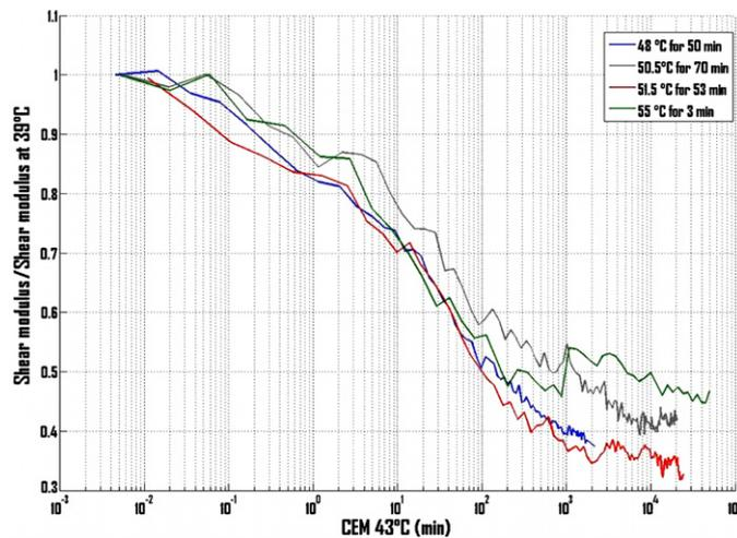
**Figure 7.** Combined influence of temperature and time for four bovine muscles: evolution of the shear modulus as a function of the cumulative thermal dose (CEM 43 °C)
