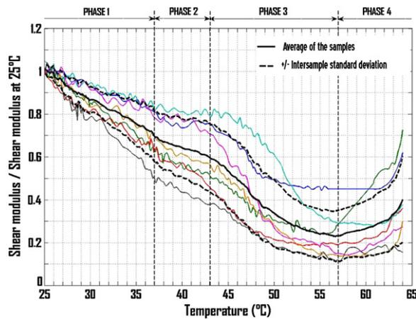
**Figure 3.** Evolution of the normalized shear modulus along the muscular fibers ('longitudinal shear modulus') during heating for seven bovine muscles. Four phases are identified: the shear modulus linearly decreases up to 43 °C with a change of slope at 37 °C (phases 1 and 2), then it exponentially decreases up to 57 °C (phase 3) and finally it exponentially increases until the end of the heating (phase 4).
