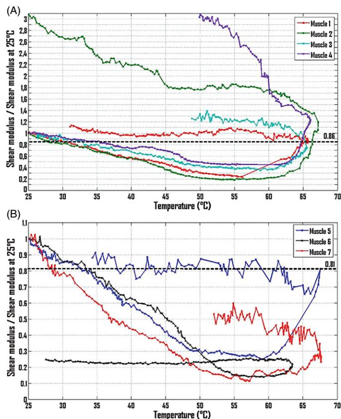
**Figure 4.** Evolution of the normalized shear modulus along the fibers during heating and cooling. (A) At the end of the heating, stiffness was bigger than 86% of the initial value: the shear modulus increased during cooling. (B) At the end of the heating, stiffness was smaller than 81% of the initial value: the shear modulus was quasi constant during cooling.
