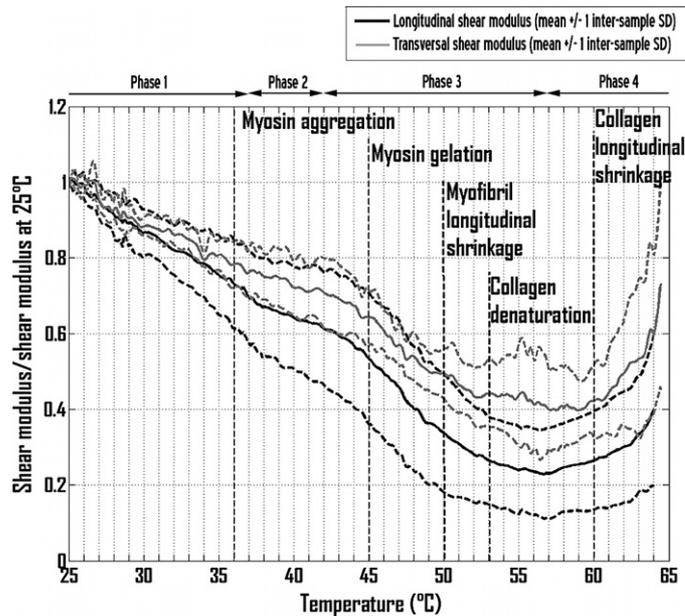
**Figure 8.** Thermal changes of the longitudinal and transversal shear moduli of bovine muscle and comparison with theoretical temperature thresholds of protein denaturation (Tornberg 2005).
