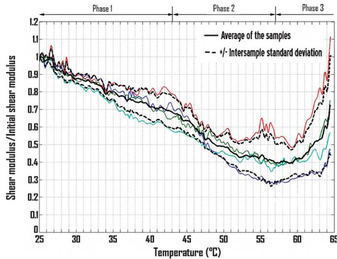
**Figure 5.** Evolution of the normalized shear modulus perpendicular to the muscular fibers ('transversal shear modulus') during heating for four bovine muscles. Three phases are identified: the shear modulus linearly decreases up to 43 °C (phase 1), then it exponentially decreases up to 57 °C (phase 2) and finally it exponentially increases until the end of the heating (phase 3).
