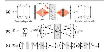
FIG. 1. (a) Schematic view of a disordered slab illuminated by a plane wave. The reflected speckle  $\mathbf{x}$  produced at the sample surface is registered on a CCD camera with N pixels, and its mutual information  $\mathcal{I}$  with the transmitted speckle  $\mathbf{y}$  is evaluated. (b) Diagrammatic representation of the trace formula (3) as a sum of correlation loops. (c) Diagrammatic representation of the approximation (6).
