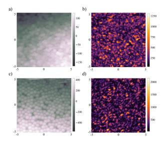
Fig. 2. Scans in contact mode for the two samples. a) Topography, and b) intensity images measured in one zone of sample A. c) and d) the same for sample B. The vertical and horizontal scales units are  $\mu$ m. Colorbars are in nm for a), c) and PM counts for b), d).
