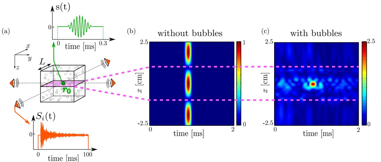
FIG. 1. (Color online) (a) A source located at  $\mathbf{r}_0$  sends a broadband wave packet in the 50–60 kHz range, and the field  $S_i(t)$  is recorded by a four-element TR mirror. (b) Back-propagated field within a line in the  $x$  direction as a function of time (b-scan), in pure liquid (no bubble). (c) The same b-scan when a  $L = 2$  cm,  $\Phi = 10^{-4}$  cloud of 50- $\mu\text{m}$ -radius bubbles is present.
