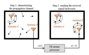
At Institut Langevin, we design original analog architectures for processing optically-carried radiofrequency signals. These architectures rely on a versatile "atomic processor" based on light-matter interaction in rare-earth ion-doped crystals cooled down to a few kelvin. In such crystals, one can make the atomic medium emit a light pulse with a controlled temporal shape by using the photon echo process. We recently proposed a modified
