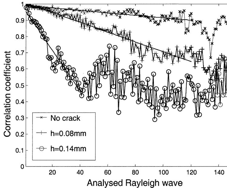
Fig. 10. Second method: comparison of two signals acquired on the same part. Acquisition time: 2 ms.
