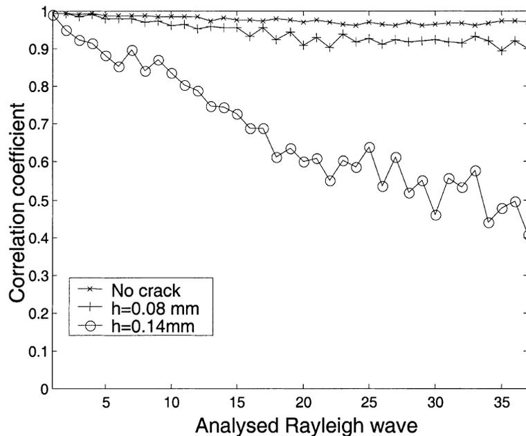
Fig. 9. Evolution of the correlation coefficient. Second method: comparison of two signals acquired on the same cylindrical part.
