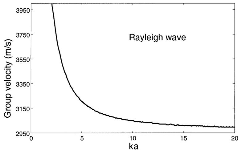
Fig. 2. Rayleigh wave dispersion curve for a steel cylinder.
