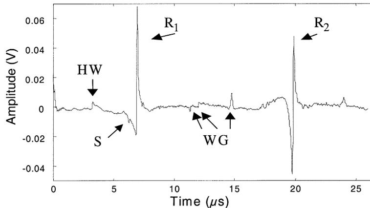
Fig. 4. Pulse waveform detected on a steel cylinder of diameter 25 mm. R refers to Rayleigh wave, HW to the head wave, WG to the whispering gallery waves and S to the shear wave.
