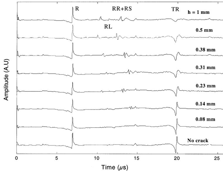
Fig. 5. Interaction of an incident Rayleigh wave (R) with slots of various depth ( $h$ ).
