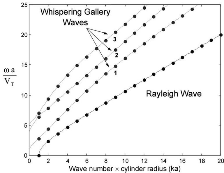
Fig. 1. Surface waves propagating on the free surface of a steel cylinder ( $V_L = 5910$  m/s,  $V_T = 3200$  m/s). The lowest curve corresponds to the Rayleigh wave, the other curves refer to whispering gallery waves. An integer value  $n$  of  $ka$  gives resonance frequency  $\omega_n$ .
