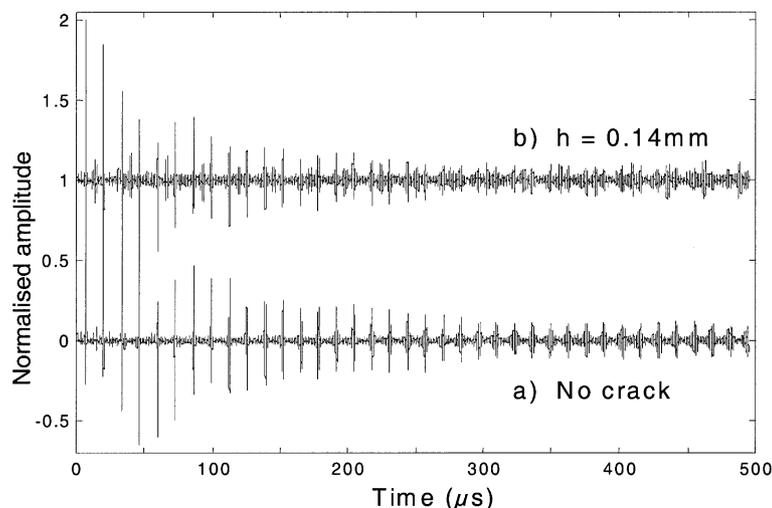
Fig. 6. Rayleigh waves on a steel cylinder of diameter 25 mm. (a) Without crack, (b) with a 0.14-mm depth slot.
