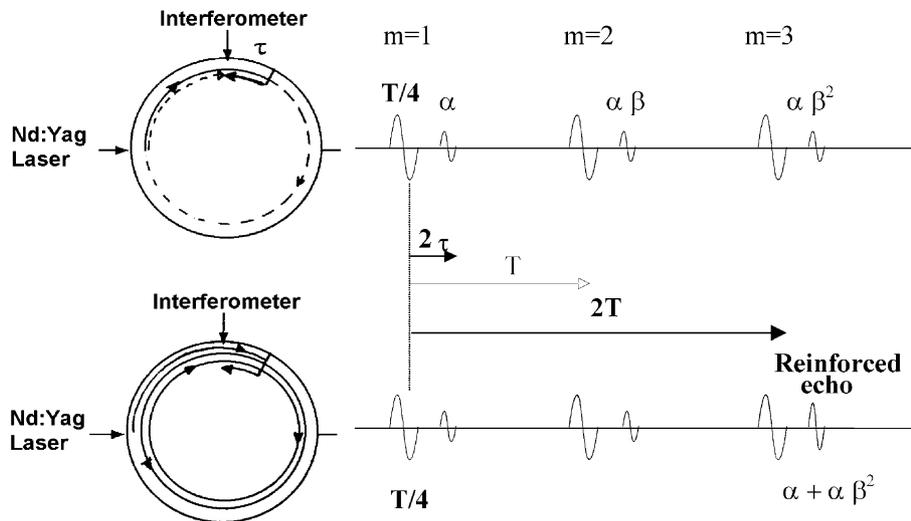
Fig. 7. Description of the cumulative effect on a cylinder.
