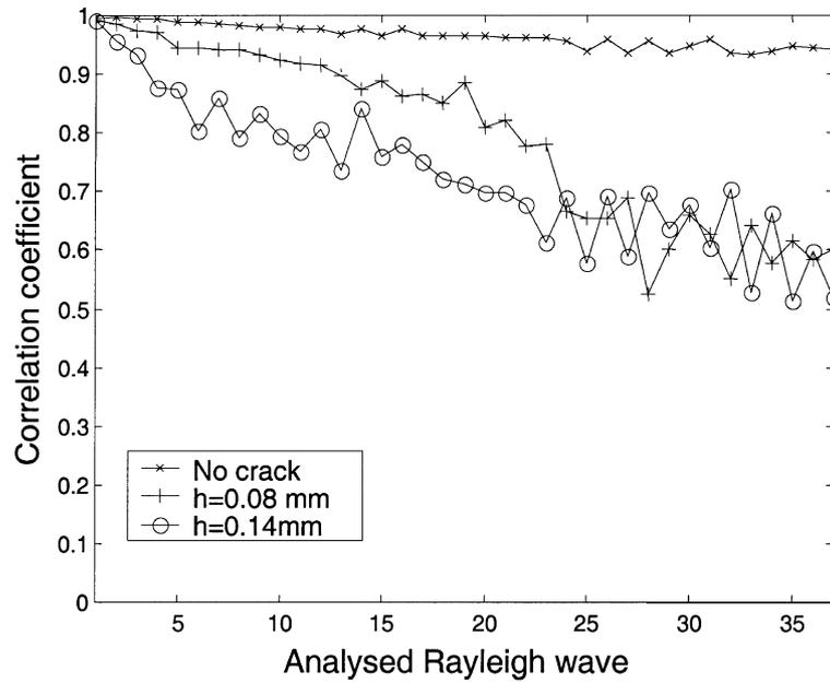
Fig. 8. Evolution of the correlation coefficient versus the analysed Rayleigh wave. First method: comparison with a reference signal.
