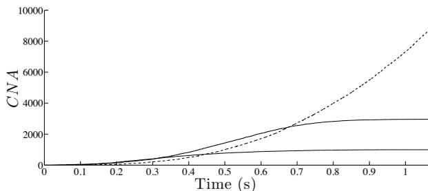
Figure 6: Cumulative numbers of the arrivals ( $CNA$ ) generated by the stochastic model of RIR (without compensation of energy decay). -dashed: model -plain: the atom is a pistol shot -bold: the atom is a dirac.
