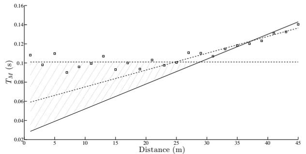
Figure 21: Mean mixing times from the model (triangles) and from the experiments (squares). Dashed lines: linear regressions made on the model (for  $d \geq 25m$ ). Plain line: linear regression of experimental RIRs. Hatched part: missing contribution of diffusion and room filtering in the model.
