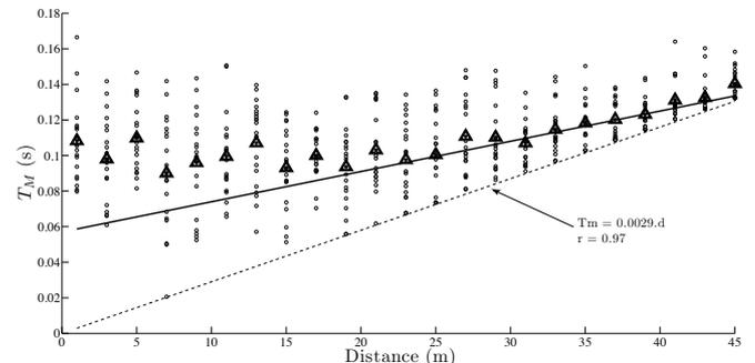
Figure 19: Mixing times (dots) detected for 20 RIRs synthesized at different distances (the time of propagation is taken into account) ( $SRR = 5dB$ ). Triangles: mean times. Dashed line: linear fit on the minima mixing times (for  $d \geq 19m$ ). Plain line: linear fit on the mean mixing times (for  $d \geq 25m$ ).
