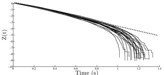
Figure 8: plain: Logarithm of  $(1 - CDF)$  of the arrivals of 21 experimental RIRs (without compensation of the energy decay) -dashed: mean logarithmic decay of the RIRs.
