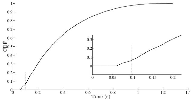
Figure 7:  $CDF$ , for an experimental RIR (without compensation of the energy decay). Dashed line: a kink in the distribution of arrivals is noticeable. The encapsuled graphic is a zoom on the early times of the  $CDF$ .
