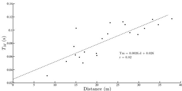
Figure 18: Estimated mixing times (dots) as a function of distance (with time propagation between the source and the receiver). Dashed line: linear regression.
