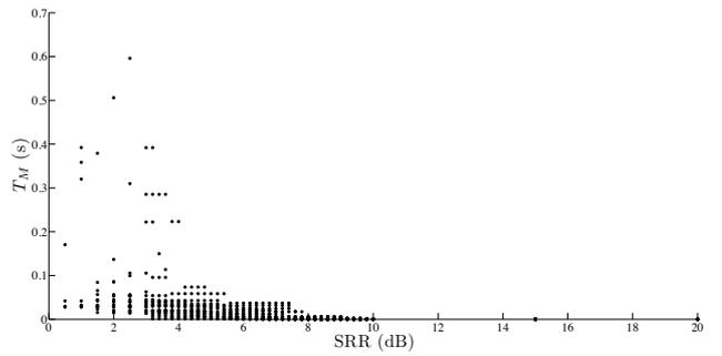
Figure 15: Mixing times estimated on experimental RIRs using different values of  $SRR$  ( $dB$ ) (compensating the energy decay).
