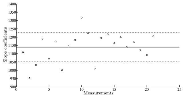
Figure 12: Circles: Slope coefficients of the linear fits made on the 21 *CNAs* ( $mean = 1140$  arrivals/second,  $std = 7.7\%$ ). Plain line: mean slope coefficients. Dashed lines: standard deviation.
