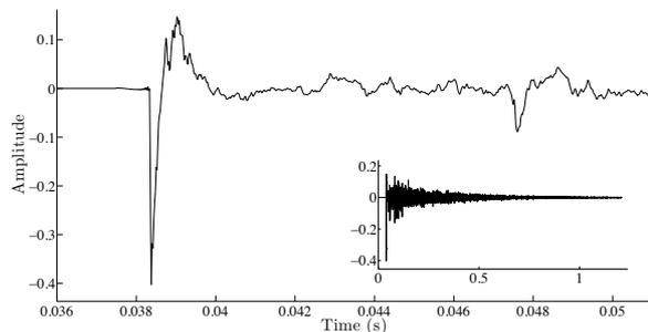
Figure 5: Detail of an experimental RIR for which determining the direct sound is not obvious.
