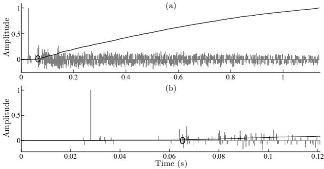
Figure 13: a): Mixing time (circle) detected on a *CDF* (bold line) for an experimental RIR and the set of estimated arrivals. ( $SRR = 5dB$ ). Plot (b) details the beginning of plot (a).
