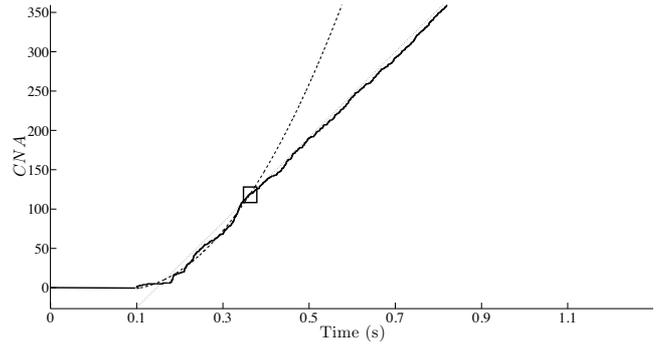
Figure 11: Detail of a cubic ( $t < T_M$ ) and a linear ( $t > T_M$ ) fits made on a *CNA*. Plain bold line: *CNA*. Dashed bold line: cubic fit. Dashed line: linear fit. Square: mixing time.
