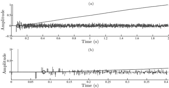
Figure 14: a): Mixing time (circle) detected on a *CDF* (bold line) for a synthesized RIR convolved with a pisol shot and the set of estimated arrivals ( $SRR = 5dB$ ). Plot (b) details the beginning of plot (a).
