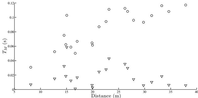
Figure 17: Estimated mixing times as a function of distance (without (triangles) and with (circles) time propagation between the source and the receiver).
