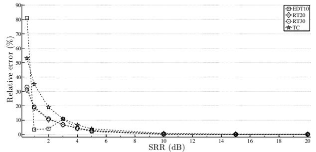
Figure 16: Variations in % of  $EDT_{10}$ ,  $RT_{20}$ ,  $RT_{30}$ ,  $T_C$  versus the  $SRR$  in  $dB$  (compensating the energy decay).
