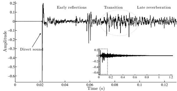
Figure 1: Early times of an experimental RIR (encapsuled graphic), measured in Salle Pleyel.
