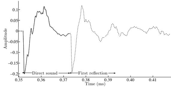
Figure 2: Experimental RIR for which determining the direct sound is obvious. Plain line: direct sound.
