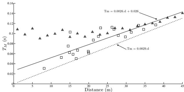
Figure 20: Mean mixing times of the model (triangles) and of the experiments (squares). Dashed line: linear regression made on the model. Plain line: linear regression of experimental RIRs.
