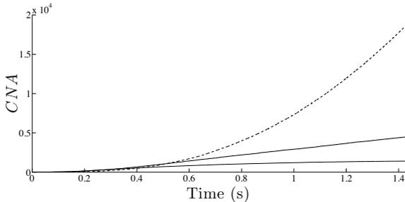
Figure 10: *CNA* of a theoretical RIR. -dash: theoretical *CNA* -plain: estimated *CNA* (the atom is a pistol shot) -bold: estimated *CNA* (the atom is a dirac) (with compensation of the energy decay).
