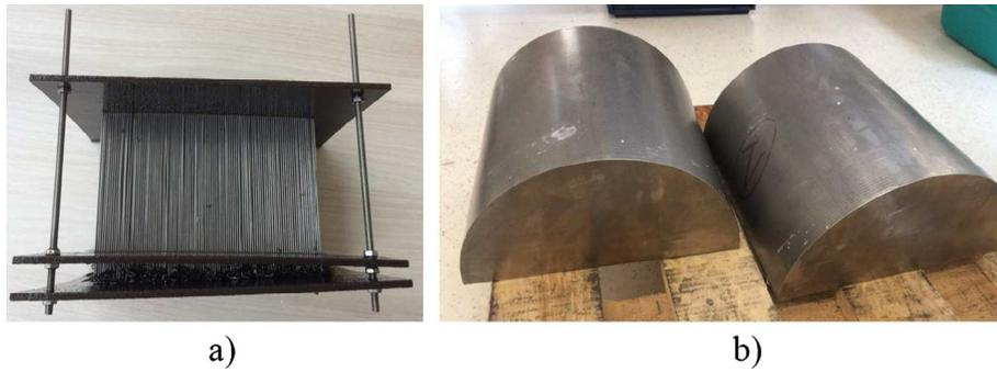
**Fig. 1.** Samples used for the experiments: (a) collection of randomly placed parallel rods called Random Rod Forest, (b) two half billets of TA6V and Ti17 titanium alloys.
