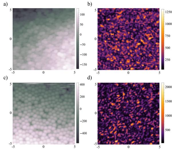
Fig. 2. Scans in contact mode for the two samples. a) Topography, and b) intensity images measured in one zone of sample A. c) and d) the same for sample B. The vertical and horizontal scales units are  $\mu\text{m}$ . Colorbars are in nm for a), c) and PM counts for b), d).
