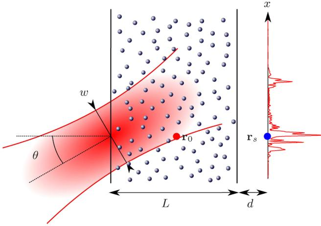
FIG. 1. (Color online) Sketch of the disordered medium. The incident Gaussian beam is focused on the input interface with an angle  $\theta$ .  $\mathbf{r}_0$  is a point inside the medium where the LDOS  $\rho(\mathbf{r}_0, \omega)$  is computed.  $\mathbf{r}_s$  is a point on the observation plane where the transmitted intensity  $I(\mathbf{r}_s, \omega)$  is computed. The red solid line is an example of speckle pattern calculated in the observation plane.
