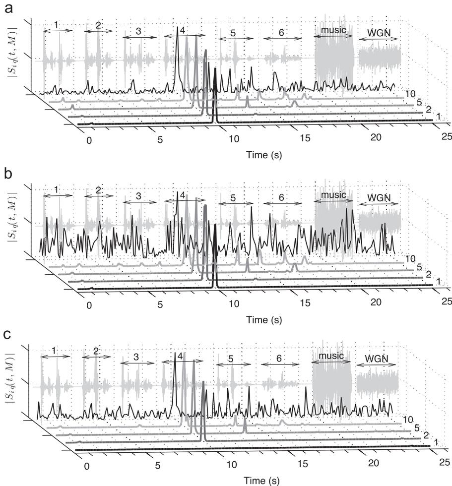
**Fig. 10.**  $|S_{iq}(M, t)|$  (28) as a function of time and the number of atoms  $M$  (labeled at right) considered from each representation for each localized sparse approximation. Localized magnitude correlation of each signal with query is shown by the thin black line in front of the gray time-domain signal at rear. (a) clean signal, (b) Signal with AWGN at 10 dB energy and (c) Signal with crow signal at 5 dB energy.
