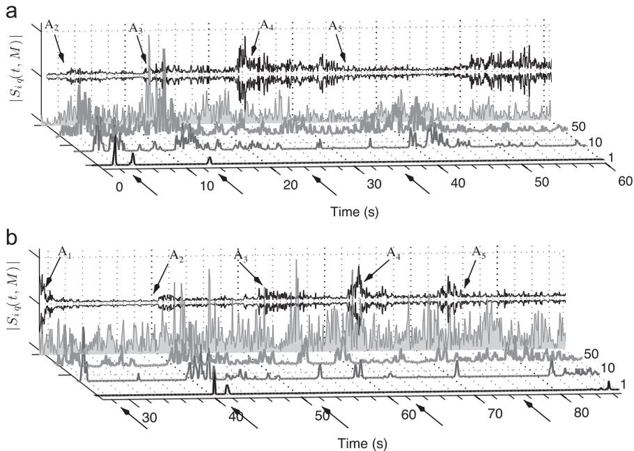
Fig. 12.  $|S_{iq}(t, M)|$  (28) for three values of  $M$  for the query and two different signals. Arrows mark the appearances of the “A” theme, and their appearance number. Magnitude correlation of query with localized and normalized signal is shown by the solid gray area in front of the black time-domain signal at rear. (a) Query compared with original signal and (b) Query compared different interpretation.
