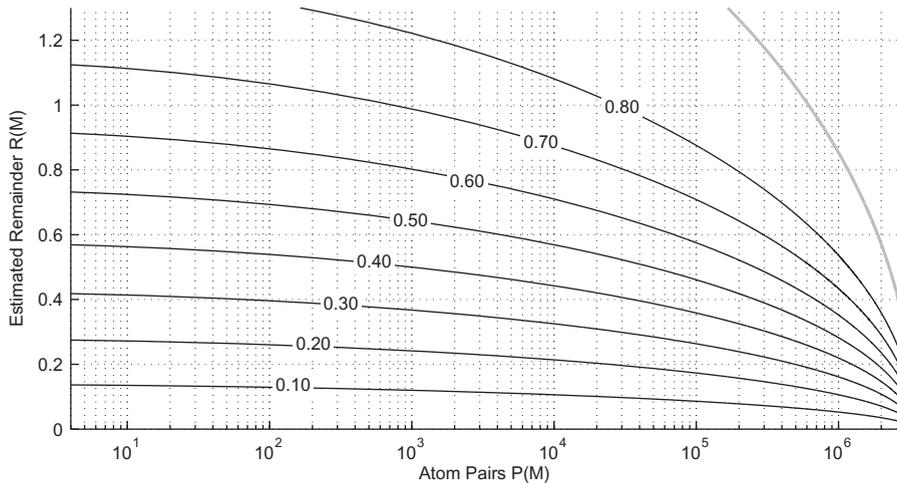
**Fig. 5.** Estimated remainder (assuming unit-norm signals) as a function of the number of atom pairs already considered for dataset used to produce Fig. 1. Gray: bound in (15). Black, numbered: bound in (16) for several labeled  $p$  (probability that remainder does not exceed bound) with  $n=2375$  (number of elements in each sparse model), and  $(C, \gamma) = (0.4785, 0.5)$ .
