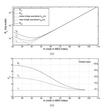
FIG. 1. Model for (a) inharmonicity coefficient  $B_{\xi}(m)$  and (b) octave type parameter  $\rho_{\phi}(m)$  along the compass for different values of the sets of parameters.
