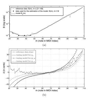
FIG. 10. RWC grand piano #1. (a) Inharmonicity curves along the compass. (b) Actual tuning and proposed tuning. Plus grey markers correspond to the data. The model corresponding to the octave type choice  $\bar{\rho}_{\phi}(m)$  (resp.  $\bar{\rho}_{\phi,L}(m)$ ,  $\bar{\rho}_{\phi,H}(m)$ ) is depicted as black line (resp. black dashed line, black dashed line with circle markers).
