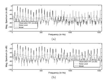
FIG. 3. (a) Initialization and (b) result of the algorithm for the analysis of F#1 note from RWC grand piano #1 database.
