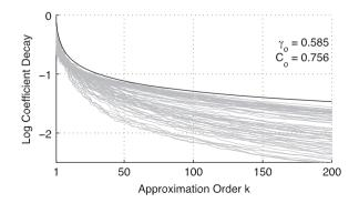
**Fig. 1.** Gray lines show decays of representation weight magnitudes as a function of approximation order k for several decompositions of unit-norm signals (4-s recordings of single piano notes described in Section 4.1). Thick black line shows a global compressibility bound with its parameters.
