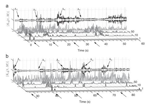
**Fig. 12.** |*S*<sub>*iq*</sub>(*t*,*M*)| (28) for three values of *M* for the query and two different signals. Arrows mark the appearances of the "A" theme, and their appearance number. Magnitude correlation of query with localized and normalized signal is shown by the solid gray area in front of the black time-domain signal at rear. (a) Query compared with original signal and (b) Query compared different interpretation.
