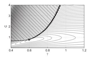
**Fig. 3.** Error surface as a function of the compressibility parameters for the dataset used to produce Fig. 1, with the feasible set shaded at top left, and optimal parameters marked by a circle.
