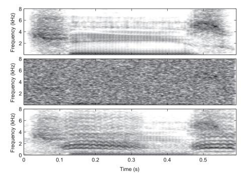
**Fig. 9.** Log spectrograms of the query signals with which we search. Top: query of male saying "cheese." Middle: query distorted with additive white Gaussian noise (AWGN) with SNR = -10 dB. Bottom: query distorted with interfering crow sound with SNR = -5 dB.
