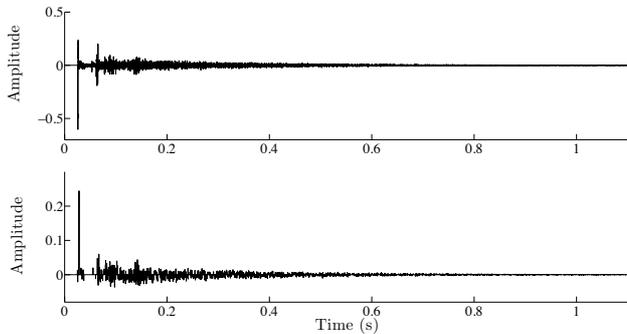
Figure 4: Matching Pursuit run on an experimental RIR ( $SRR = 20dB$ ). -(top): Experimental RIR -(bottom): Linear set of coefficients, which correspond to the arrivals.
