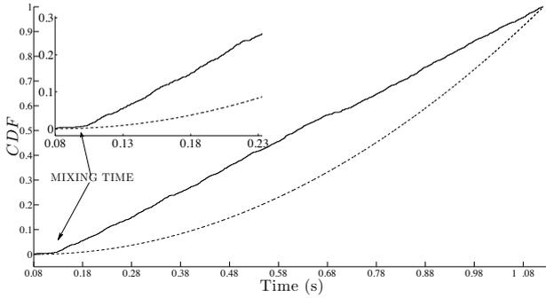
Figure 9: *CDFs*. -dash: theoretical *CDF* ( $\approx t^3$ ) -plain: Average of *CDF* for 21 RIRs (with compensation of the energy decay). The encapsuled graphic is a detail of the early part of the *CDF*.
