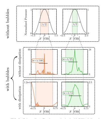
FIG. 5. (Color online) Focal spots obtained with BW1 (left) and BW2 (right) in three configurations: in pure water (top), in a  $\Phi = 0.01$  bubble cloud with no dissipation (middle), and in the same cloud with dissipation (bottom). The bubble cloud is a 1-cm-edge cube. Fields are normalized by the maximum of pressure obtained in the absence of bubbles.
