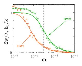
FIG. 4. (Color online) Dimensionless FWHM  $2w/\lambda$  as a function of gas volume fraction  $\Phi$  (symbols), compared to the dimensionless effective wavelength  $k_0/k$  predicted by the ISA (lines).
