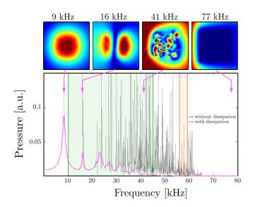
FIG. 6. (Color online) Pressure spectra obtained at one point of the z = 0 section of a  $\Phi = 0.01$  bubble cloud with (thick pink line) and without (thin black line) dissipation. Edges of the cubic cloud are 1 cm long. Insets on the top are 2D field maps at different frequencies (represented by pink arrows) within the z = 0 section, in the case of bubbles with dissipation.
