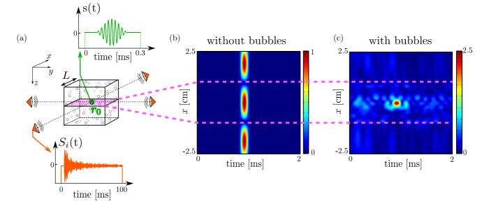
FIG. 1. (Color online) (a) A source located at  $\mathbf{r}_0$  sends a broadband wave packet in the 50–60 kHz range, and the field  $S_i(t)$  is recorded by a four-element TR mirror. (b) Back-propagated field within a line in the *x* direction as a function of time (b-scan), in pure liquid (no bubble). (c) The same b-scan when a L = 2 cm,  $\Phi = 10^{-4}$  cloud of 50- $\mu$ m-radius bubbles is present.
